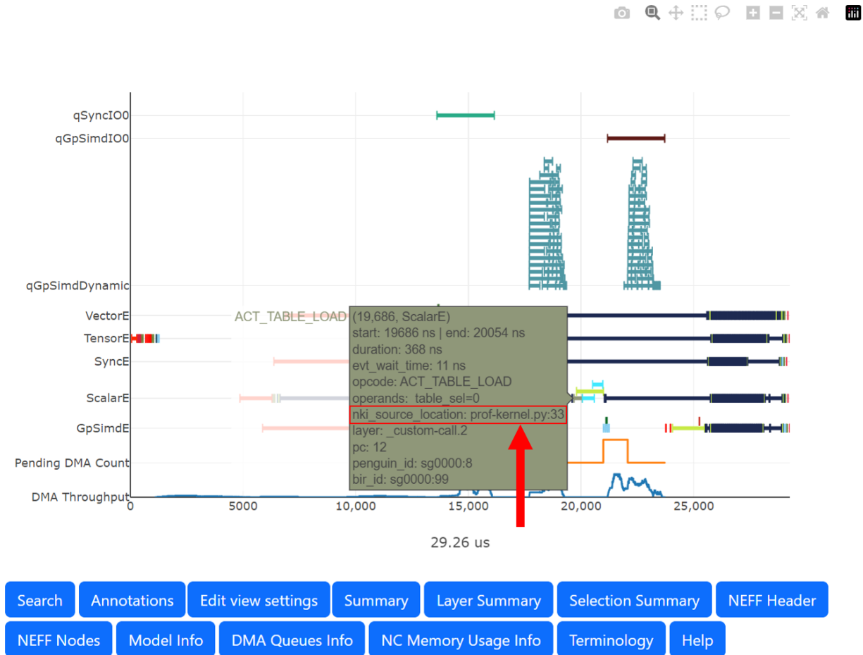
Fig. 7.29: Instruction hover details including the line of NKI source code that generated this instruction.
