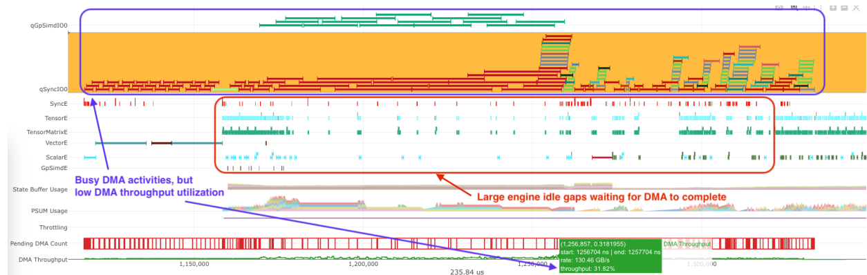
Fig. 7.61: Busy DMA engines with relatively idle compute engines.
