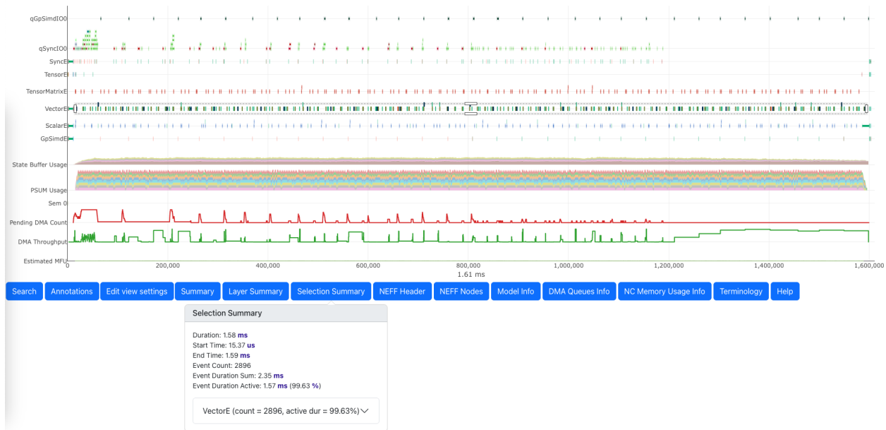
Fig. 7.94: Profile of mamba_v2 kernel with loop reordering optimization
