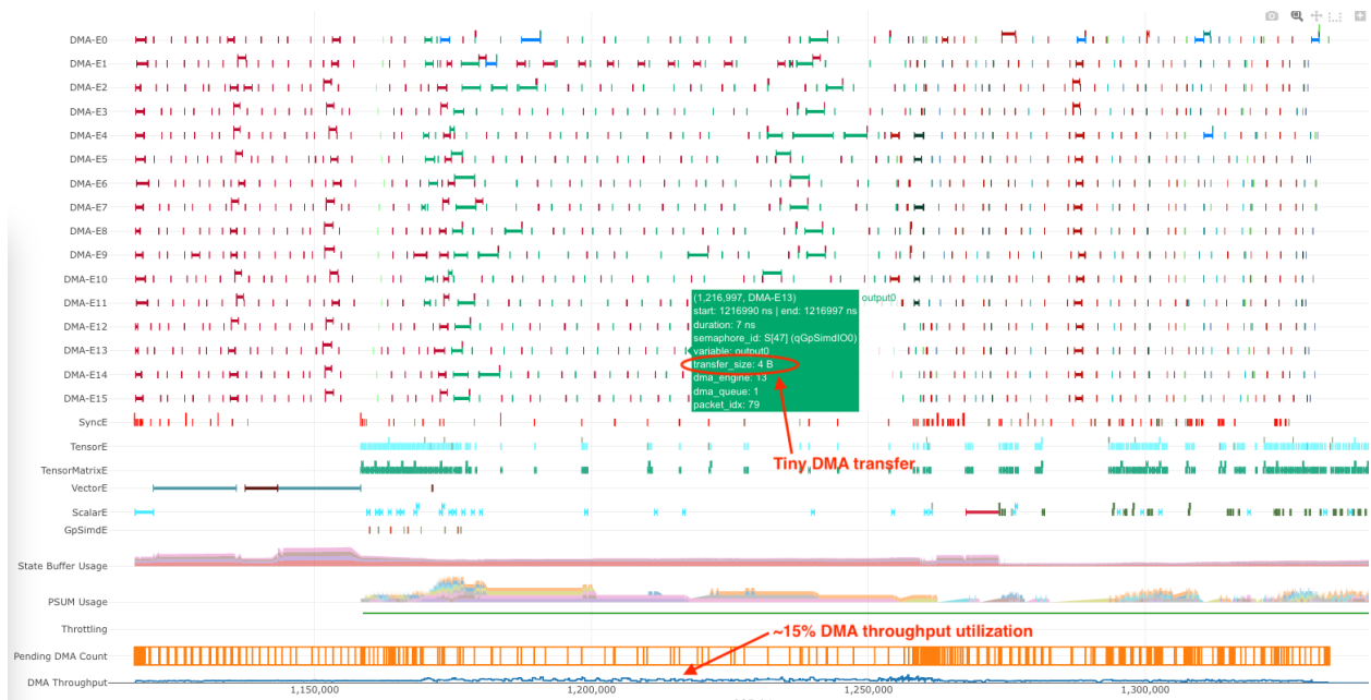
Fig. 7.63: Example timeline with tiny DMA transfers.
