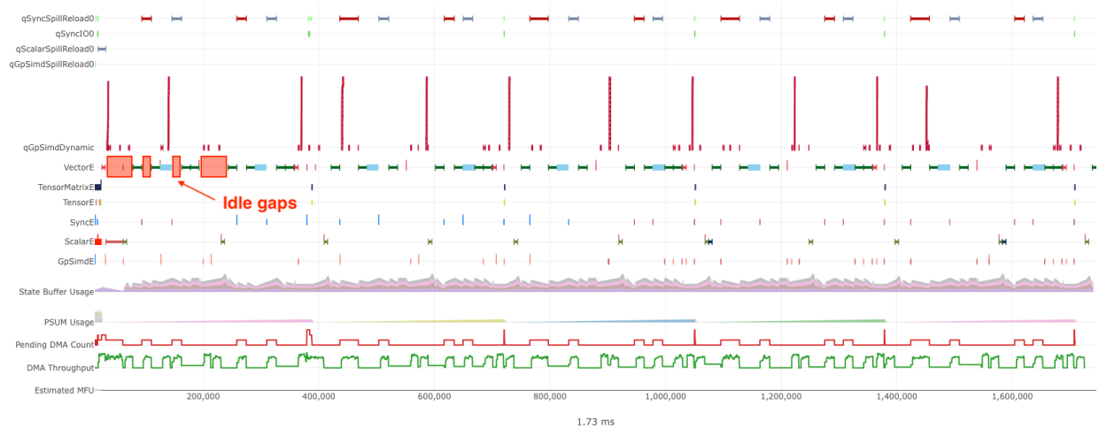
Fig. 7.43: Engine idle gaps.
