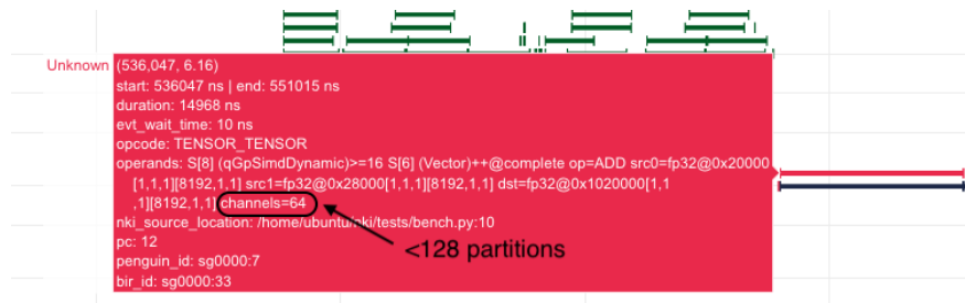
Fig. 7.52: An instruction that read/write less than 128 partitions.
